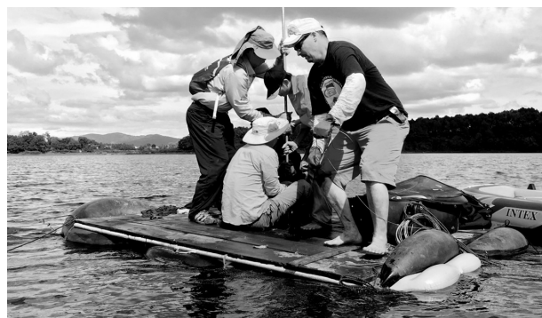
Fig. 2 - Gravity and piston coring in November 2017 on an improvised platform on Biển Hồ maar lake from water depths up to ~21 m.
